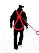
Fall FACTOR 2 anchor point located below the back anchor point of the harness
