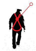
Fall FACTOR 0 Anchor point located above the head
